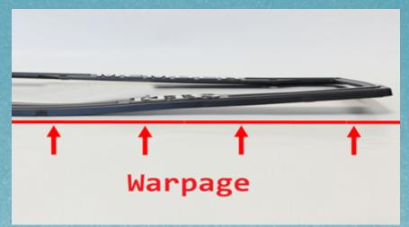
There are multiple parameters that lead to warpage in any plastic injection moulded part and these may vary depending on various conditions like type of polymer used, melt temperatures, injection pressures etc. These simulation softwares help to understand the actual deformation or warpage in any injection moulded part thus saving time and increasing efficiency. Design engineers and manufacturers should make use of softwares more to avail its benefits.
