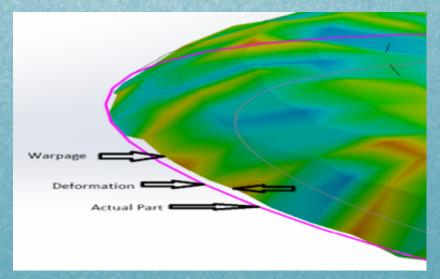
Deformation due to warpage is observed in all the three directions (X,Y,Z).
