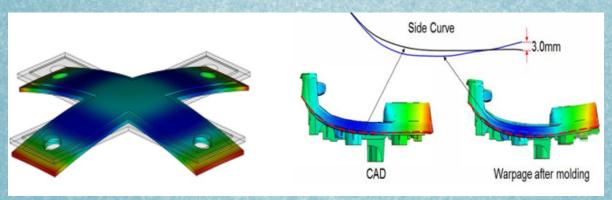
Simulation on 'Solid works Plastics' showing deformation in the y direction.
