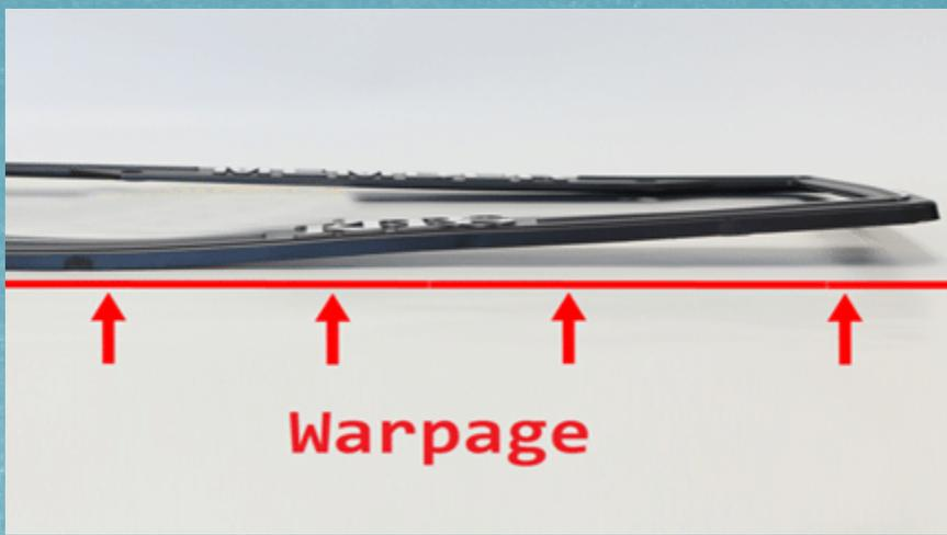
There are multiple parameters that lead to warpage in any plastic injection moulded part and these may vary depending on various conditions like type of polymer used, melt temperatures, injection pressures etc. These simulation softwares help to understand the actual deformation or warpage in any injection moulded part thus saving time and increasing efficiency. Design engineers and manufacturers should make use of softwares more to avail its benefits.
