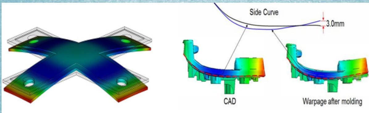
*Simulation on 'Solid works Plastics' showing deformation in the y direction.*
