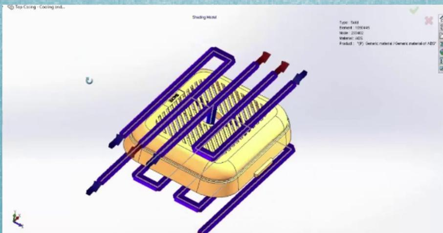
*Addition of cooling channels to minimize part warpage*
